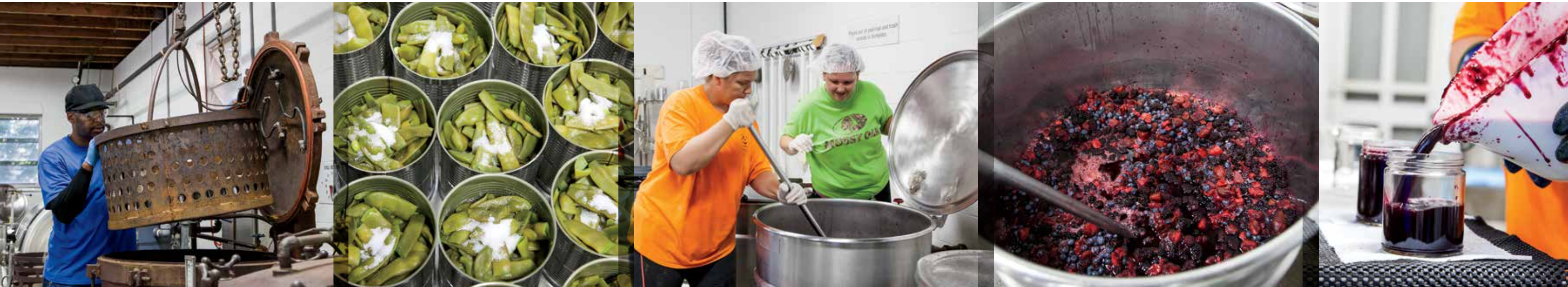
Far left: Cannery assistant, Rodney Scott, lowers cans into the retort for pressure cooking. Center left: Steamed beans await lids before processing. Center of page: Melissa Reamer
